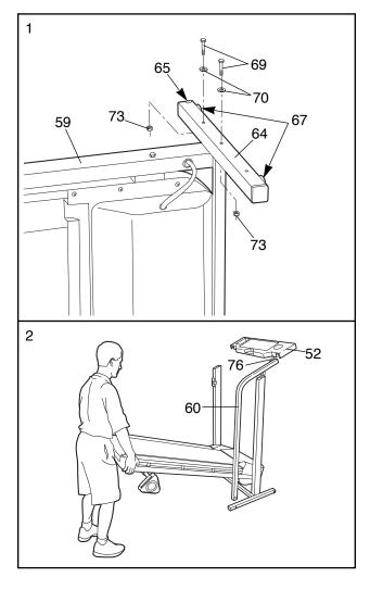
Insert the bracket on the Left Handrail (61) into the left Upright (59). While a second person holds the Console Base (52), carefully insert the Right Handrail (60) into the right Upright (59). Make sure that the lower ends of the Handrails (61, 60) are on the inside of the Base Legs (64) (refer to the inset drawing).
